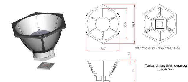
In order to determine if the particular beam properties and performance of this optic are suitable for your application with your chosen LED type, POL suggests that you obtain samples from POL or their distributors for your own product testing, as properties may vary with different LED types.
