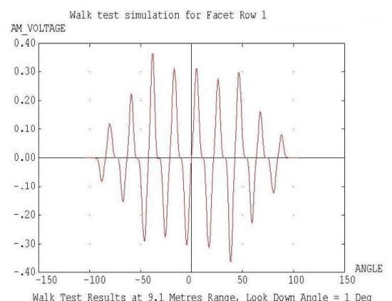
Ray-traced signal plot simulation
