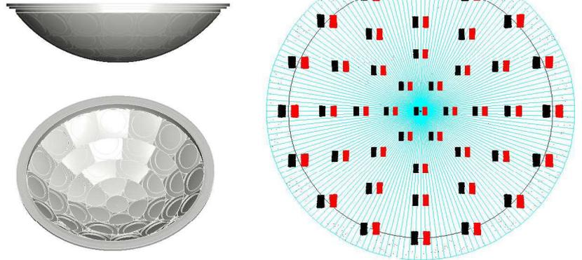
Suppose we were to design a similar lens with a flat profile. Traditional technology dictates that we use circularly symmetric Fresnel facets using diamond turning and wire-eroding tool construction methods. The ray-traced zone plot shows how the outer zones have become unacceptably distorted.
