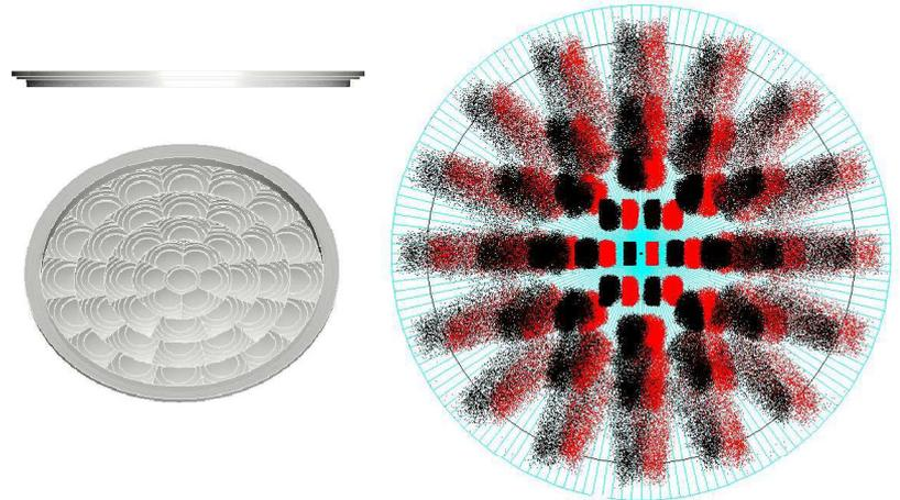
Now however we have developed the software to design Free-form fresnel lenses that give very low distortion. The free-form design on the right has been ray-traced and the plot shows that the zones are once again sharply focused, with very little distortion.
