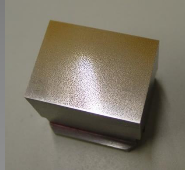
Laser Patterned Tool Insert 10cm 2 - approx. 40K dots!
