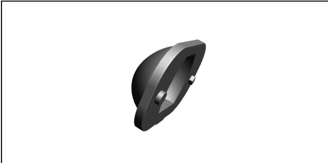
The optic is located on the PCB using a diamond dowel inserted in to a 2.5mm diameter hole and a peg in to a 3mm diameter hole. The distance between the two hole centres required is 20mm. (See dimensional drawing overleaf).
